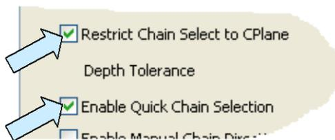
With Restrict Chain Select to Cplane and Enable Quick Chain Selection enabled in TOOLS/OPTIONS/POSITIONING SELECTION/SELECT, you can move your cursor over the profile and the entire profile will highlight. Click to accept it. Then, click on the inward-facing vector.
