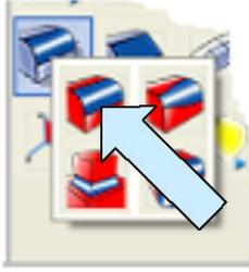
To complete your project, you can use the CONSTANT RADIUS BLEND tool with a radius of 0.05 to add blends at the root of each mounting ear and at the root of each cylindrical port.
