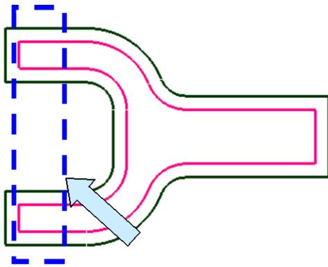
Drag a selection box around the two left ends of the smaller wishbone profile. (Do NOT include the ends of the larger profile!)
