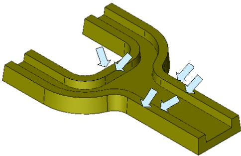
Create 0.125 radius blends on the top edges of the part indicated by arrows in the illustration to the left.
